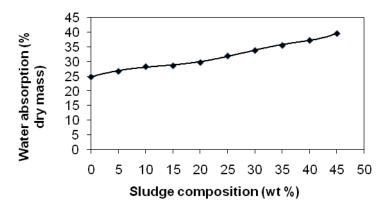
Figure 1: Effect of sludge composition on the water absorption of bricks Linear firing shrinkage
