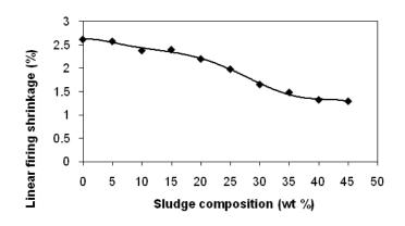
Figure 2: Effect of sludge composition on linear firing shrinkage Weight loss on ignition
