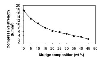
Figure 4: Effect of sludge composition on compressive strength
